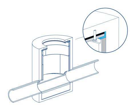
The segment rings should end about 5-10 centimeters below the old cone. Use the different heights of the segment elements (100, 250, 500 mm) to minimize the need for adjustments to the components.
