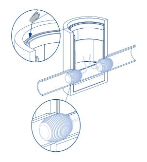
When the backfill material is completely hardened, the balloons can be removed. If a chemically resistant backfill material is used, no further actions are required. If a non-resistant backfill material is used, ensure that all the backfill surfaces are covered with DURA.Glue or an equivalent chemically resistant material to avoid any future damages to the system.
