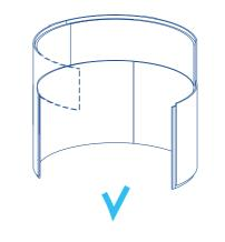
The last ring segment row will need to be cut-to-size on site, depending on the alignment. After measurement of the required height, the last ring segment row is taken out of the manhole and cut on site. Care has to be taken that the required safety measures are taken.
