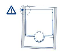
Note that in depending on the berm height, inlets or outlets might be blocked. At these points, the elements need to be cut to ensure that the connections remain open and accessible. If the berm is not blocking any inlets or outlets, the berm covers the complete circumference of the manhole, which allows for an easy alignment
